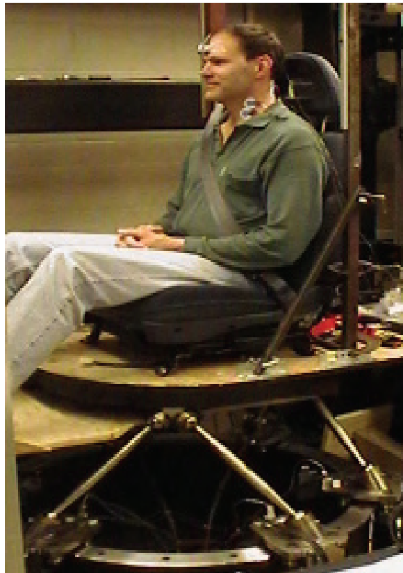
Fig. 2. Experimental setup showing a subject sitting on the automobile seat mounted to the top platform of the parallel robot. Surface EMG and head accelerometer data was collected during the perturbations with the subject secured in the car seat using the standard safety seat belt and head restraint.
