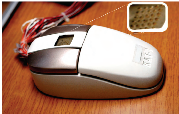
Fig. 3. A prototype of the texture display mouse
